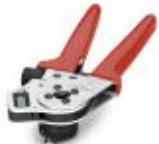
Crimping pliers for turned crimp contacts Ø 0.6 mm / Ø 0.8 mm / Ø 1 mm / Ø 2 mm, litz wire cross section of 0.06 mm<sup>2</sup> ... 2.5 mm<sup>2</sup>
