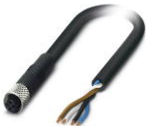
Sensor/Actuator cable, 4-position, PUR, black RAL 9005, free cable end, on Socket straight M5, A-coded, Cable length: 1.5 m
