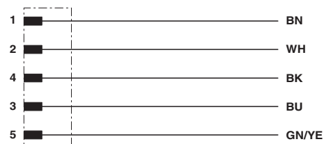
Contact assignment of the M12 plug
