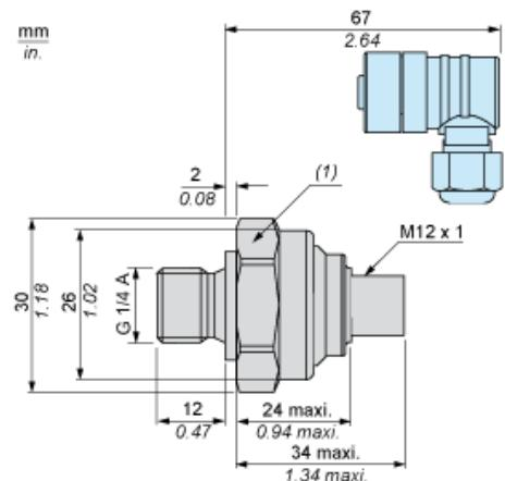
(1) SW27 Tightening torque  $\leq$  25 Nm / 221 Lb-in
