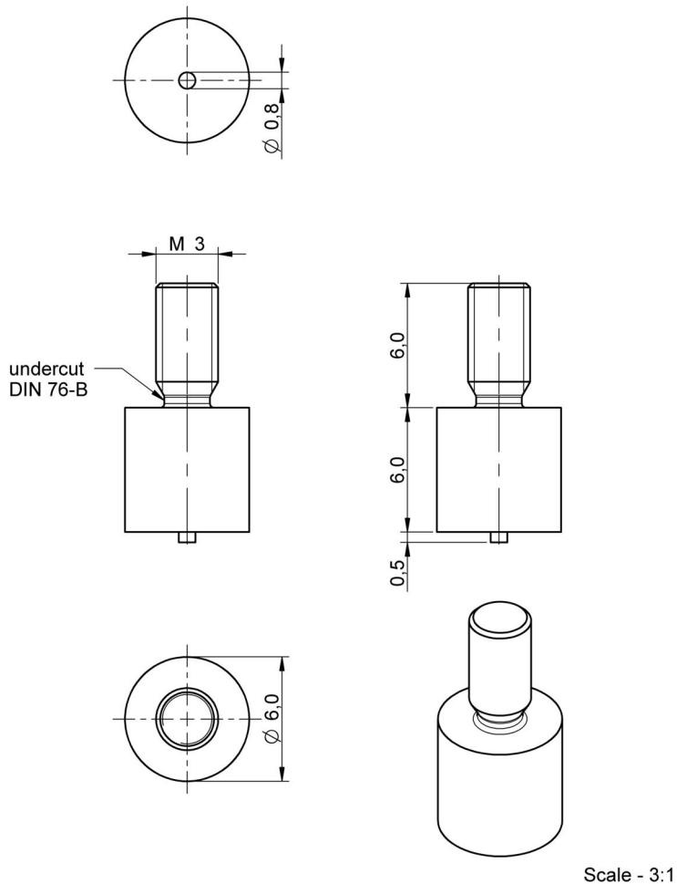
Technical Tolerances according to DIN ISO 2768m
