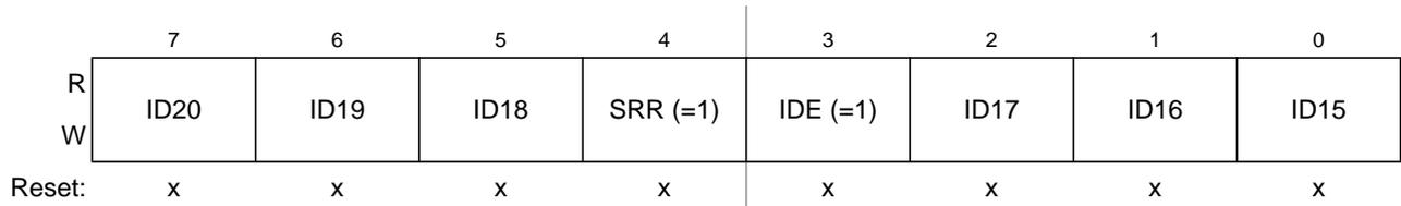
Figure 8-27. Identifier Register 1 (IDR1) — Extended Identifier Mapping
