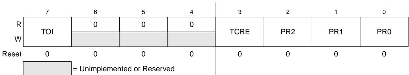
Figure 14-19. Timer System Control Register 2 (TSCR2)
