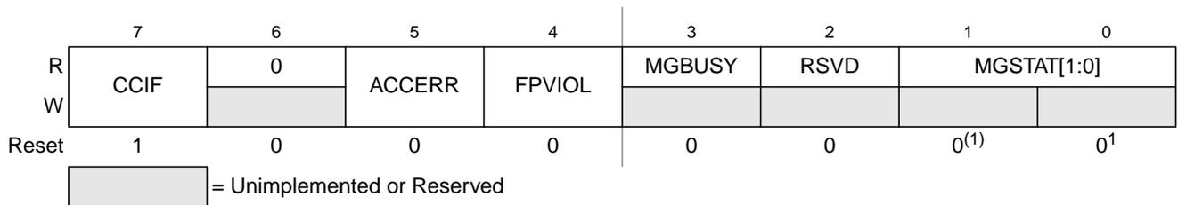
**Figure 13-11. Flash Status Register (FSTAT)**
