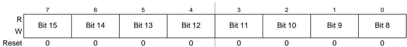
Figure 6-21. Debug Comparator Data High Mask Register (DBGADHM)
