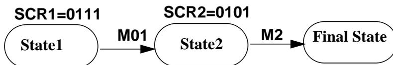
A trigger is generated if a given sequence of 2 code events is executed, whereby the second event is entry into a range (COMPA,COMPB configured for range mode)
