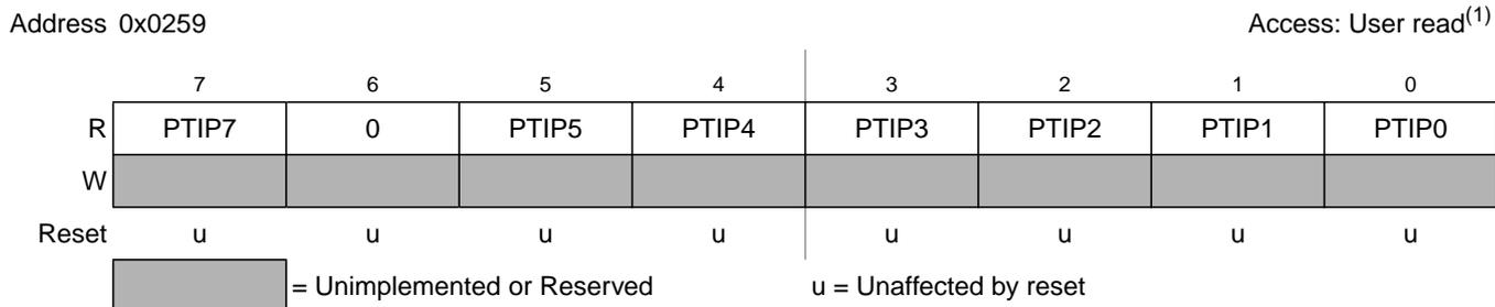
**Figure 2-39. Port P Input Register (PTIP)**
