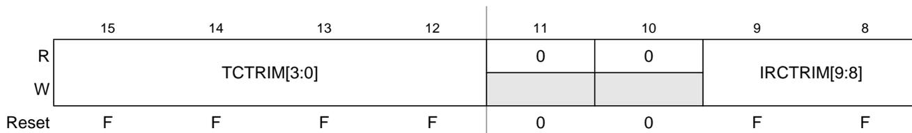
After de-assert of System Reset a factory programmed trim value is automatically loaded from the Flash memory to provide trimmed Internal Reference Frequency  $f_{IRC1M\_TRIM}$ .
