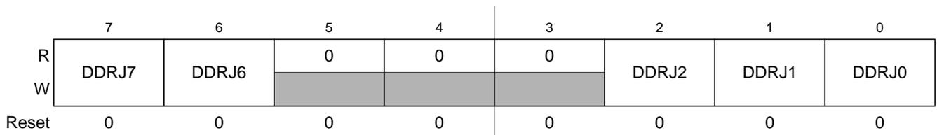
**Figure 2-49. Port J Data Direction Register (DDRJ)**
