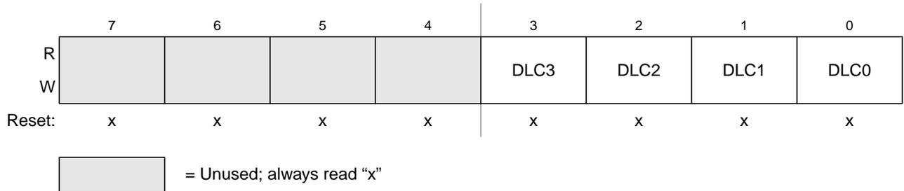
Figure 8-35. Data Length Register (DLR) — Extended Identifier Mapping
