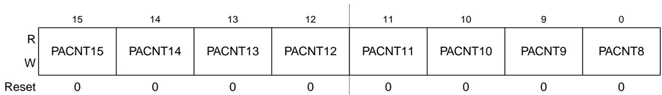
Figure 14-26. Pulse Accumulator Count Register High (PACNTH)
