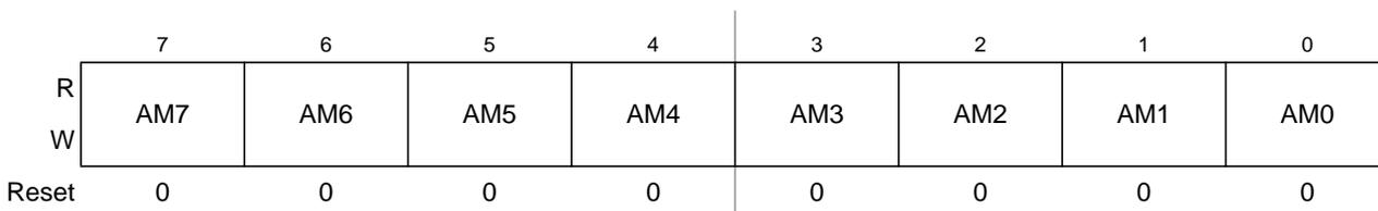
**Figure 8-22. MSCAN Identifier Mask Registers (First Bank) — CANIDMR0–CANIDMR3**
