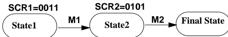
A trigger is generated if a given sequence of 2 code events is executed, whereby the first event is entry into a range (COMPA,COMPB configured for range mode). M1 is disabled in range modes.
