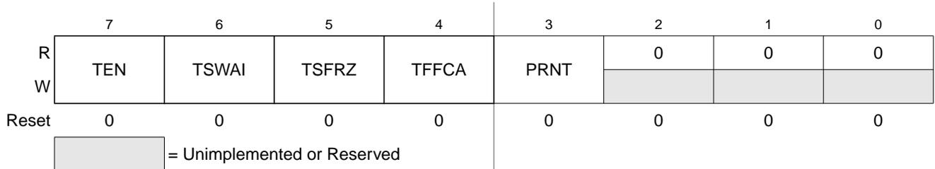
Figure 14-12. Timer System Control Register 1 (TSCR1)
