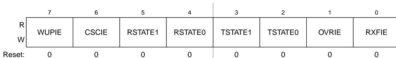
**Figure 8-9. MSCAN Receiver Interrupt Enable Register (CANRIER)**
