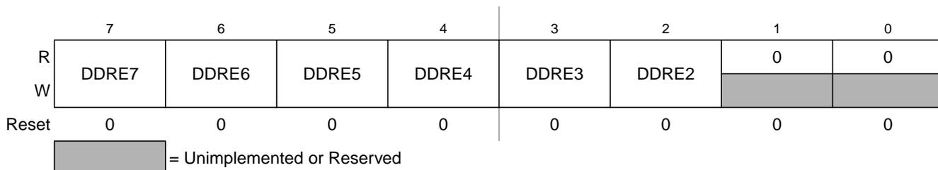
**Figure 2-7. Port E Data Direction Register (DDRE)**
