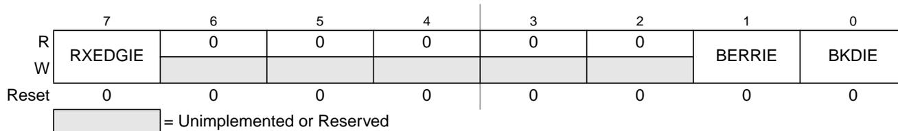
Figure 11-7. SCI Alternative Control Register 1 (SCIACR1)
