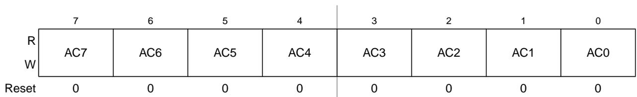
**Figure 8-21. MSCAN Identifier Acceptance Registers (Second Bank) — CANIDAR4–CANIDAR7**
