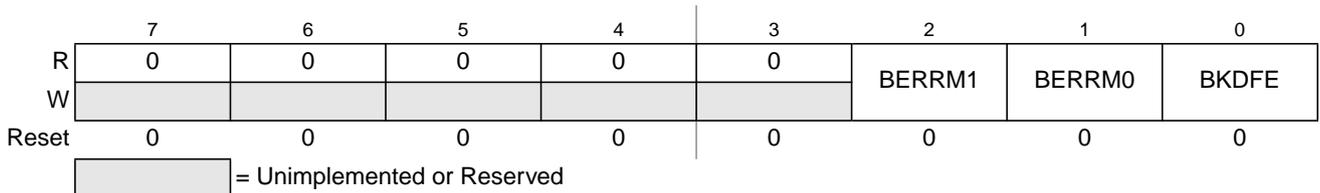
Figure 11-8. SCI Alternative Control Register 2 (SCIACR2)
