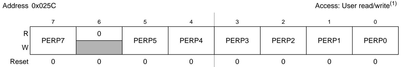
Figure 2-42. Port P Pull Device Enable Register (PERP)
