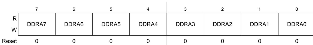
Figure 2-3. Port A Data Direction Register (DDRA)
