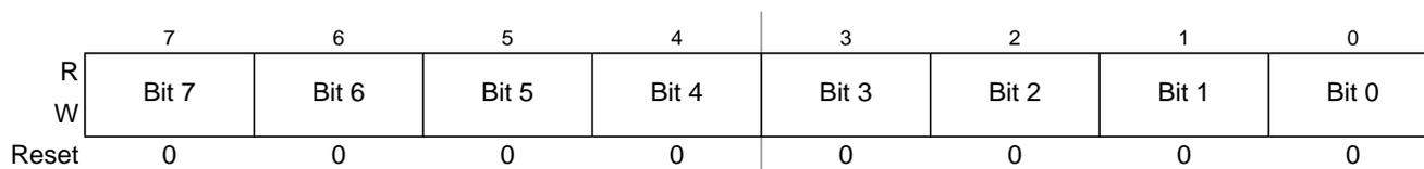
Figure 6-22. Debug Comparator Data Low Mask Register (DBGADLM)
