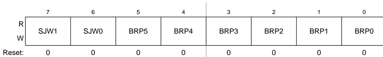
**Figure 8-6. MSCAN Bus Timing Register 0 (CANBTR0)**
