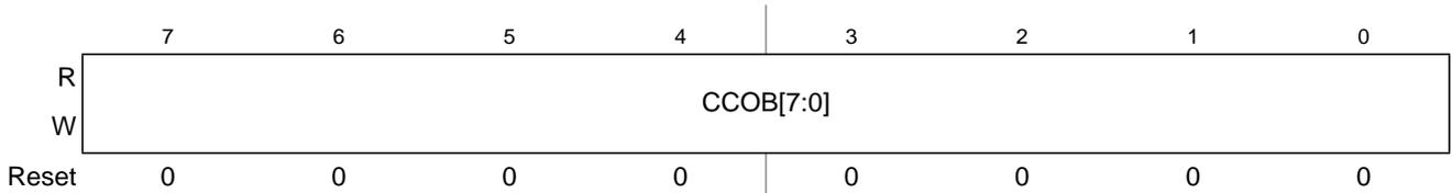
Figure 13-17. Flash Common Command Object Low Register (FCCOBLO)
