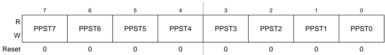
Figure 2-19. Port T Polarity Select Register (PPST)
