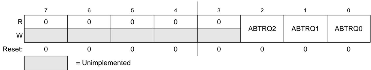
**Figure 8-12. MSCAN Transmitter Message Abort Request Register (CANTARQ)**
