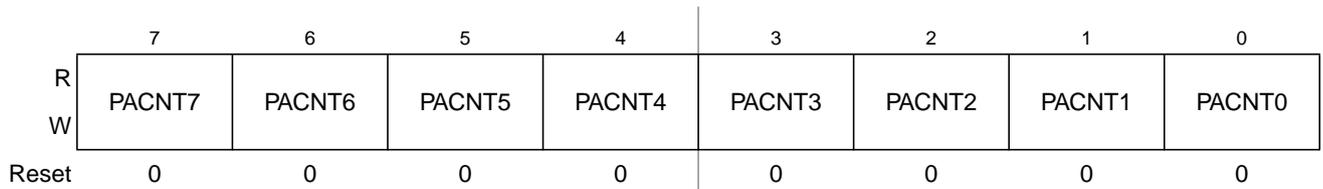
Figure 14-27. Pulse Accumulator Count Register Low (PACNTL)
