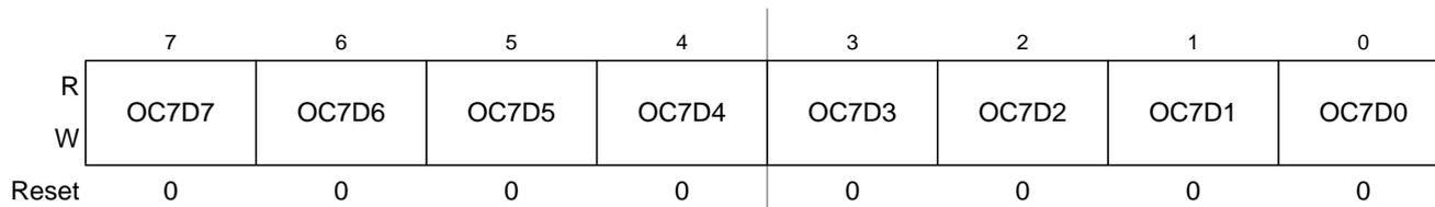
Figure 14-9. Output Compare 7 Data Register (OC7D)
