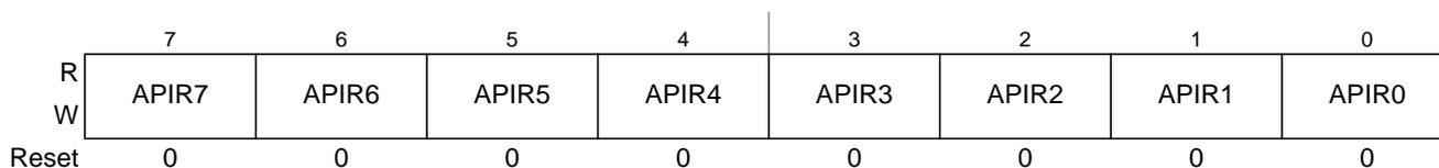
**Figure 7-22. Autonomous Periodical Interrupt Rate Low Register (CPMUAPIRL)**
