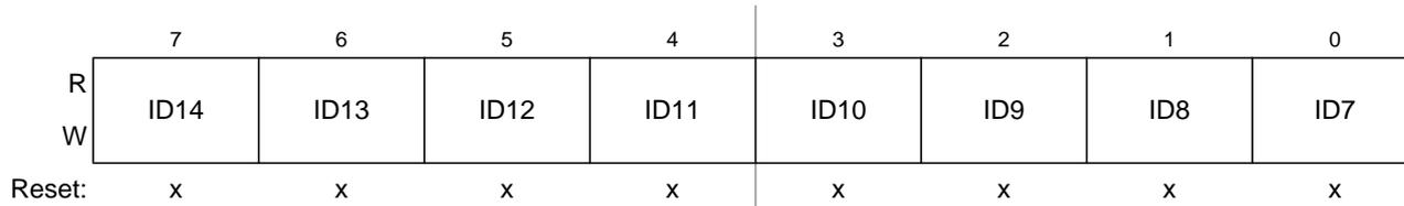
Figure 8-28. Identifier Register 2 (IDR2) — Extended Identifier Mapping
