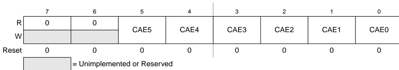
**Figure 10-7. PWM Center Align Enable Register (PWMCAE)**
