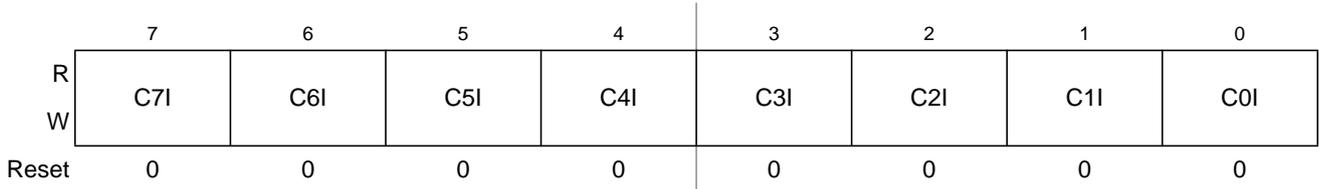
Figure 14-18. Timer Interrupt Enable Register (TIE)
