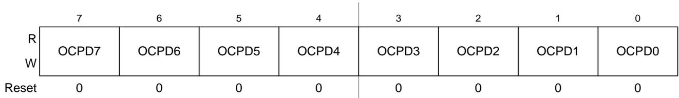
Figure 14-28. Ouput Compare Pin Disconnect Register (OCPD)
