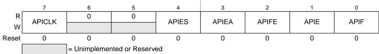
**Figure 7-18. Autonomous Periodical Interrupt Control Register (CPMUAPICTL)**
