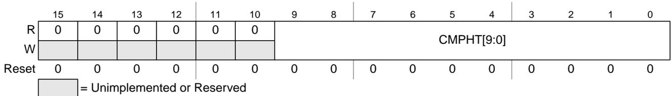
Figure 9-13. ATD Compare Higher Than Register (ATDCMPHT)
