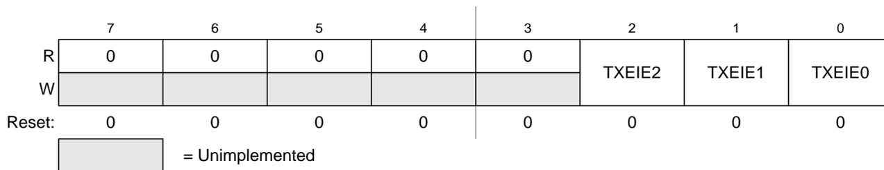
**Figure 8-11. MSCAN Transmitter Interrupt Enable Register (CANTIER)**
