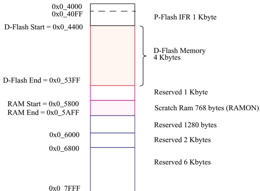
Figure 13-3. D-Flash and Memory Controller Resource Memory Map
