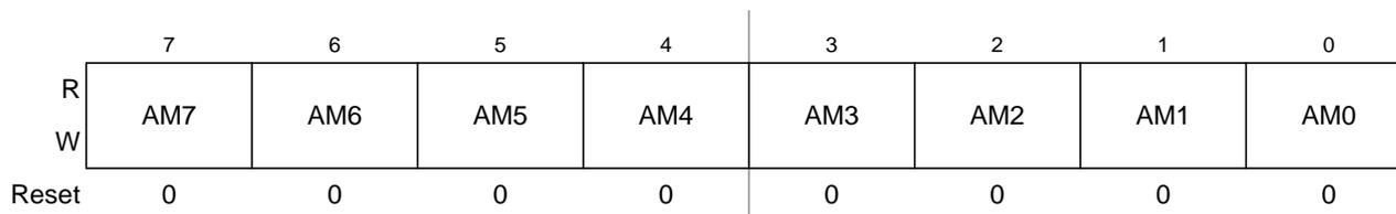
**Figure 8-23. MSCAN Identifier Mask Registers (Second Bank) — CANIDMR4–CANIDMR7**
