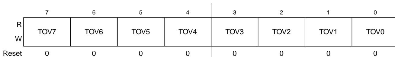
**Figure 14-13. Timer Toggle On Overflow Register 1 (TTOV)**
