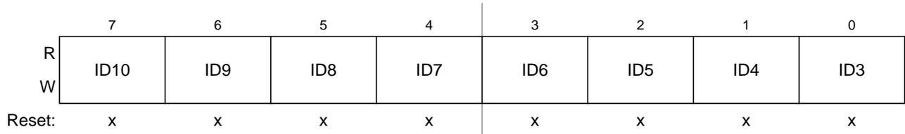
Figure 8-30. Identifier Register 0 — Standard Mapping
