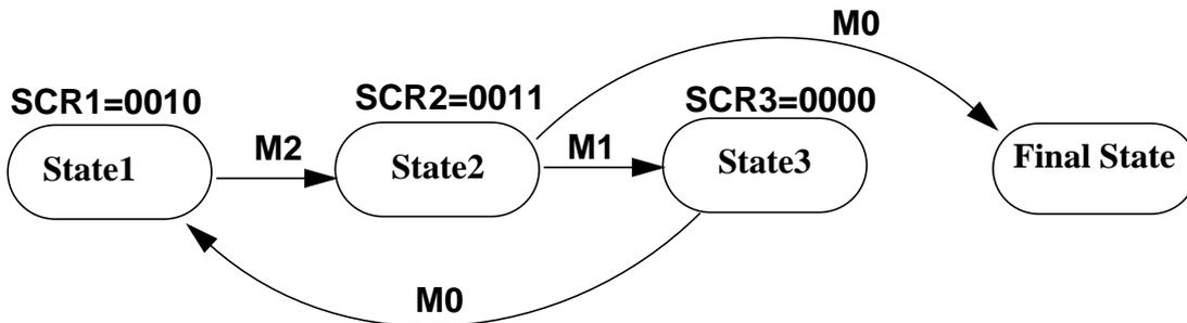
Scenario 10b shows the case that after M2 then M1 must occur before M0. Starting from a particular point in code, event M2 must always be followed by M1 before M0. If after any M2, event M0 occurs before M1 then a trigger is generated.
