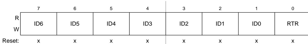
Figure 8-29. Identifier Register 3 (IDR3) — Extended Identifier Mapping
