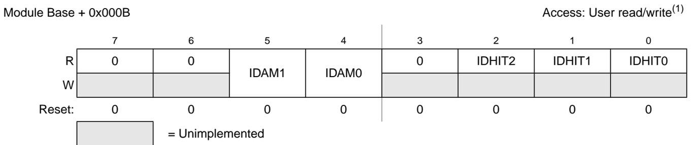
**Figure 8-15. MSCAN Identifier Acceptance Control Register (CANIDAC)**
