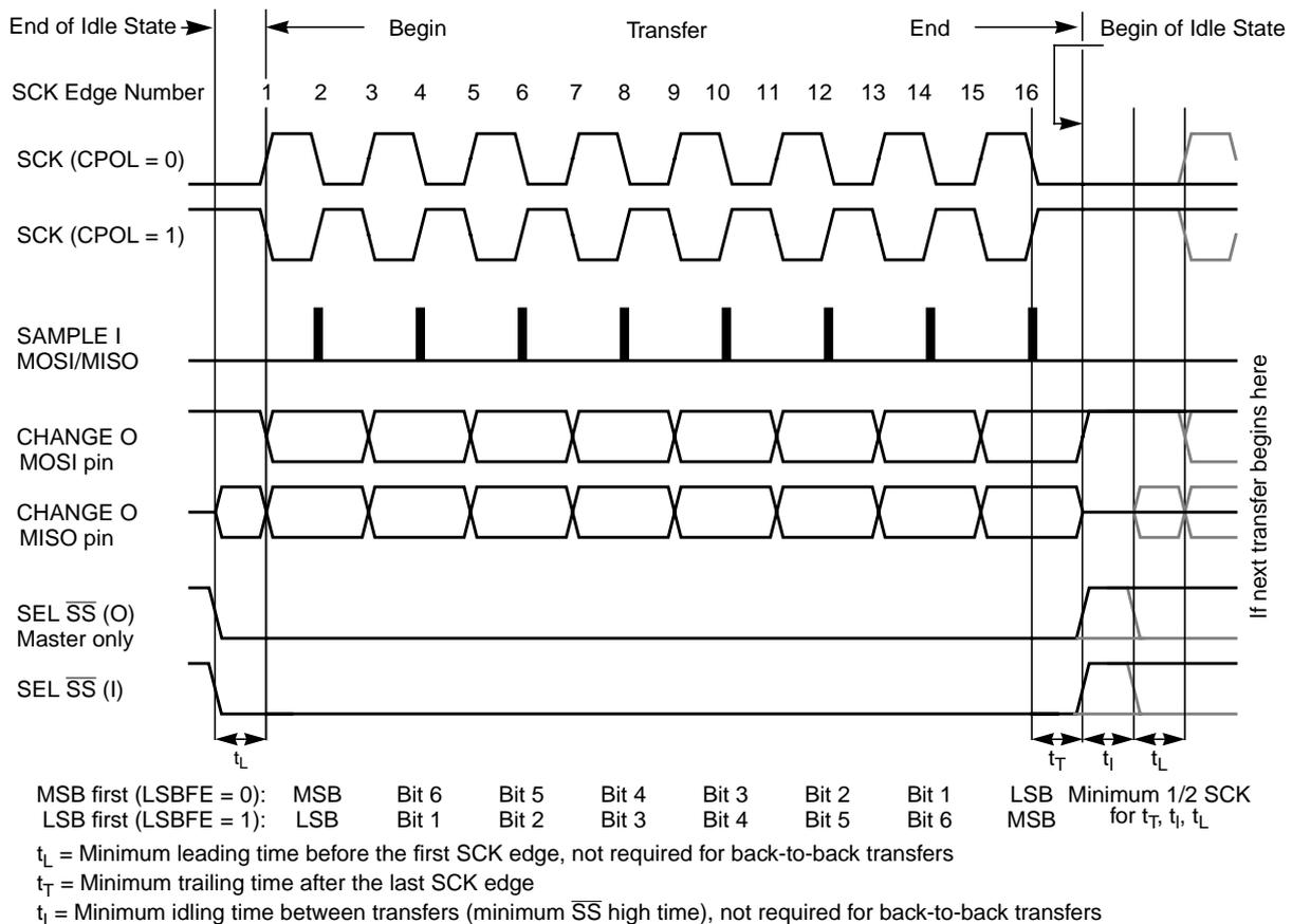
Figure 12-14. SPI Clock Format 1 (CPHA = 1), with 8-Bit Transfer Width selected (XFRW = 0)
