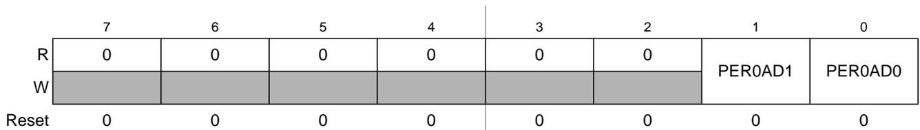
Figure 2-61. Port AD Pull Up Enable Register (PER0AD)
