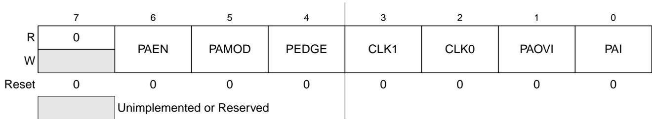
**Figure 14-24. 16-Bit Pulse Accumulator Control Register (PACTL)**
