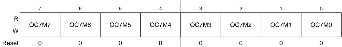
**Figure 14-8. Output Compare 7 Mask Register (OC7M)**
