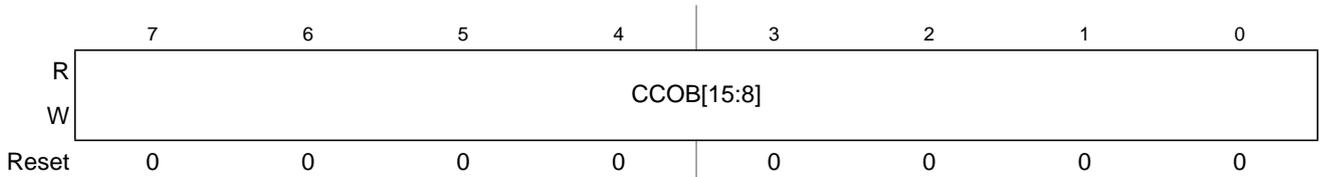
Figure 13-16. Flash Common Command Object High Register (FCCOBHI)
