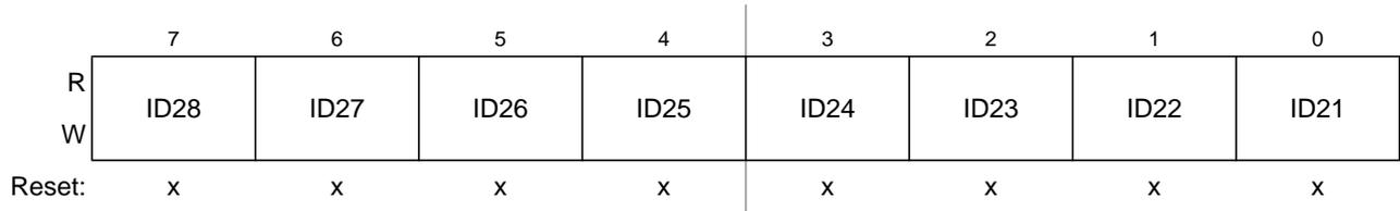
Figure 8-26. Identifier Register 0 (IDR0) — Extended Identifier Mapping
