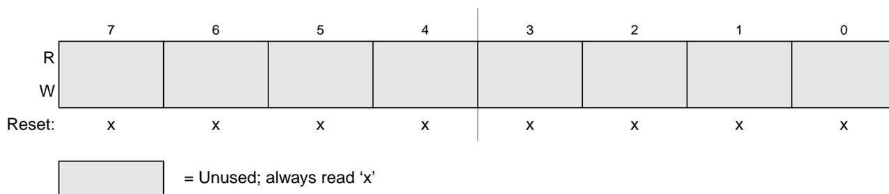
Figure 8-32. Identifier Register 2 — Standard Mapping
