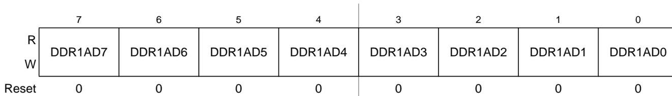
Figure 2-58. Port AD Data Direction Register (DDR1AD)
