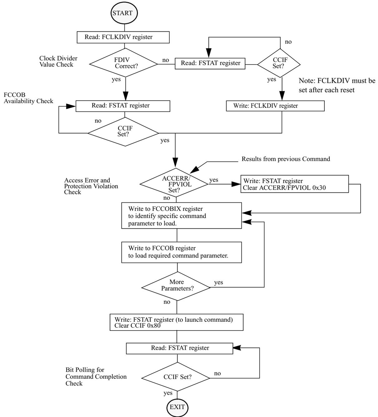
Figure 13-26. Generic Flash Command Write Sequence Flowchart
