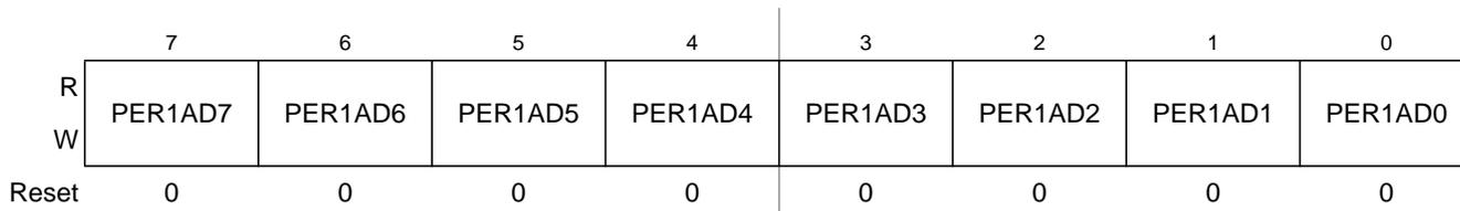
Figure 2-62. Port AD Pull Up Enable Register (PER1AD)
