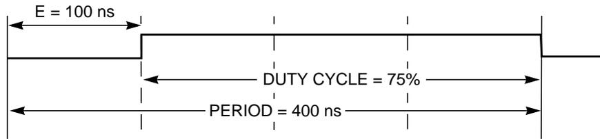
Figure 10-37. PWM Left Aligned Output Example Waveform
