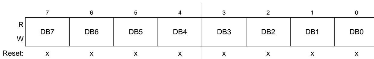
Figure 8-34. Data Segment Registers (DSR0-DSR7) — Extended Identifier Mapping
