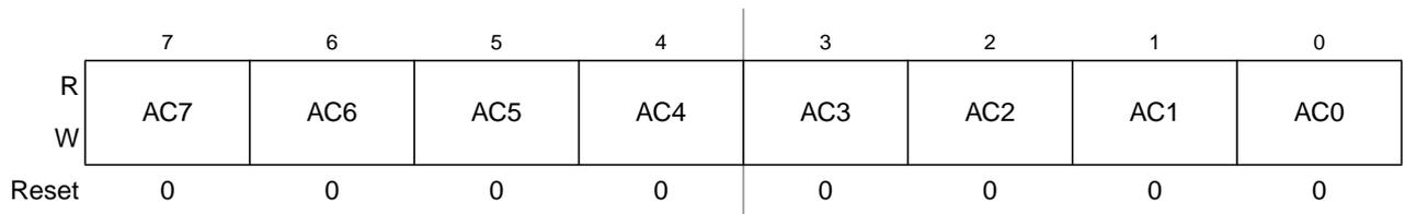
**Figure 8-20. MSCAN Identifier Acceptance Registers (First Bank) — CANIDAR0–CANIDAR3**
