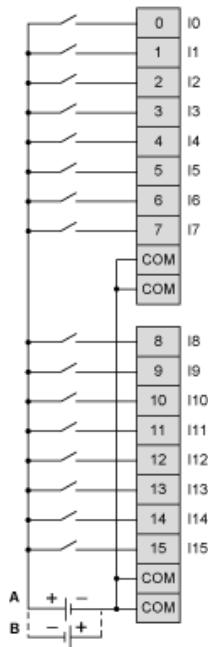
The 4 COM terminals are connected internally
