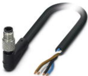
Sensor/Actuator cable, 4-position, PUR, black RAL 9005, Plug angled M5, A-coded, on free cable end, Cable length: 1.5 m
