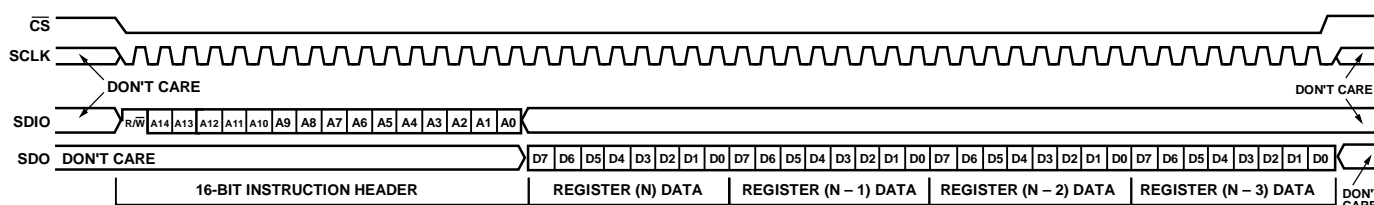
Figure 38. Serial Control Port Read—MSB First, Address Decrement, Four Bytes of Data
