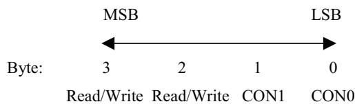
The Hitag 1 configuration bytes control whether the memory blocks are read/write or locked for read only access. Note that bytes 2 and 3 of the configuration page are not used and are currently available for general read/write use.
