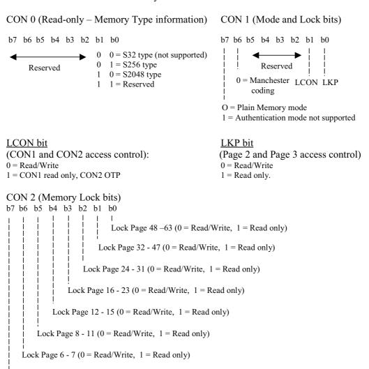
Note that CON2 (Memory Lock bits) are OTP (One-Time-Programmable) if LCON = 1 Note also that the "Reserved" bits must not be altered. Page 1 must be read first and the bits that can be changed masked on/off before writing back.
