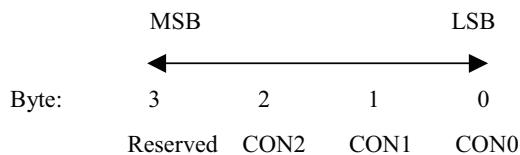
The Hitag S configuration bytes indicate the type of HS transponder and the mode of operation. Please note that the MicroRWD H1/S module only supports Plain Memory mode (default mode as set by Philips). Configuration bytes also control whether the memory blocks are read/write or locked for read only access.
